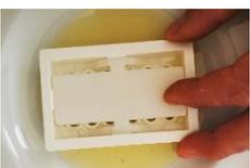
**4.** Heat the sealing solution to about 30 to 33 degrees until it is liquid. Make sure, that the solution does not get too hot, otherwise the capsules may melt. Then pour the sealing solution into a shallow bowl until it covers it to a height of about 3 mm. Press upper part into the solution for a short moment.
