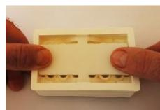
**5.** Remove the base part from the stand, place it on a flat surface and put the top part on the base part. Then press down firmly on the sides of the top part until the machine stands on the floor. The filled capsules are now automatically joined together and held in the upper part.
