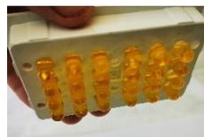
**6.** Take the upper part with the filled capsules and hold it over the drying tray. Press the white plastic plate with both hands. If the capsules do not fall out immediately, you can remove the spring plate and press the capsules from the inside out with the tamper so that they are ejected into the drying tray.
